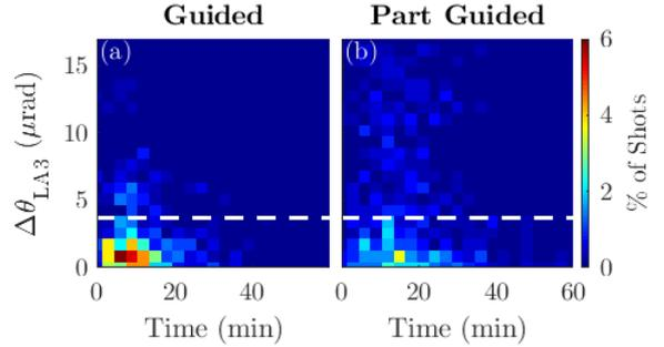
Figure 4: Histograms showing how the guided (a) and partially guided (b) shots were distributed with respect to the pointing jitter observed in LA3 ( $y$ -axis) and gradual spatial drift observed in both LA3 and TA3 ( $x$ -axis).
