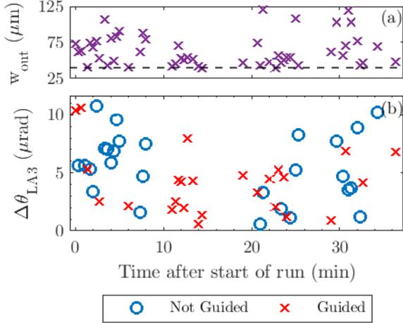
Figure 3: (a) Variation in the guided spot size  $w_{out}$ . (b) Graph showing how guiding quality is correlated with time and the LA3 leakage position for 50 consecutive shots.
