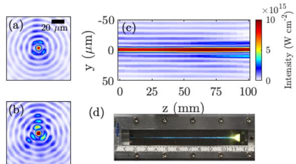
Figure 2: (a) Transverse intensity profile of the channel-forming beam at the start of the line focus. (b) Transverse intensity profile 100 mm downstream. (c) Horizontal slices of the measured transverse intensity taken at 5 mm intervals. (d) SLR image of a hydrogen plasma column ionised by the channel-forming beam.
