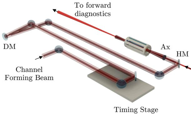
Figure 1: Interaction point setup in TA3. The channel-forming is reflected by a deformable mirror (DM), is coupled into the interaction line by a holed mirror (HM) and focussed into the gas cell by an axicon lens (Ax). The F/40 pulse is focussed to the entrance of the 100 mm gas cell containing hydrogen gas, and guided by the plasma channel to the exit.
