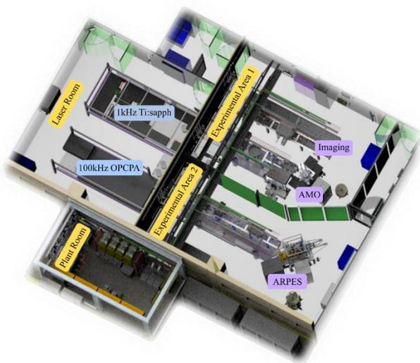
Figure 1. Schematic of the new Artemis facility in the Research Complex.
