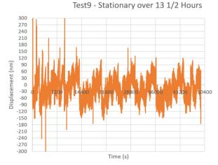
Figure 11: A 13.5 hour test showing stability before the motion control was tuned (30 nm =  $0.1 \mu$ rad)
