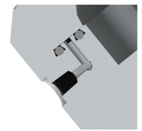
Figure 4: Cross-section through differentially pumped seal
