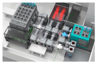
Figure 1: Multiple mirrors used in Experiment Area 2 (EA2) to propagate two beams from the compressor through various systems into the target chamber
