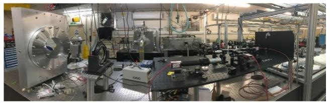
Figure 9: Optical setup test, the positioning mirror is on the left hand side
