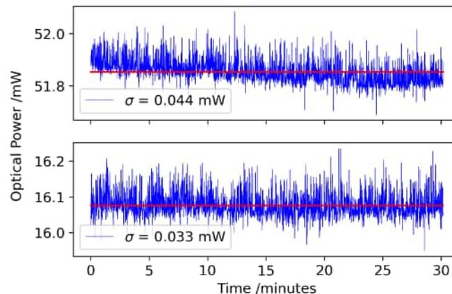
Figure 7: (Top) Input optical power measured over 30 minutes, (Bottom) Output optical power measured over 30 minutes.
