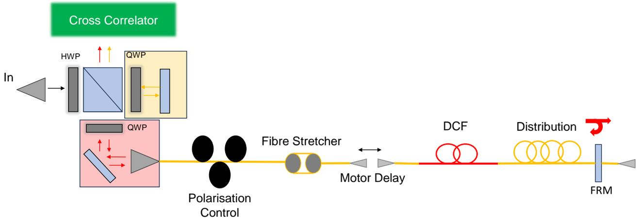
Figure 1: Single mode stabilised fibre optic link including an in line polarisation controller, fibre stretcher for fast stabilisation, motor delay to keep the stretcher within range, dispersion compensating fibre (DCF) to maintain short pulse duration at the output of the link and a Faraday rotator mirror (FRM) before the output. Light reflected from the FRM travels back through the link into a cross-correlator where a path-length sensitive signal is generated.
