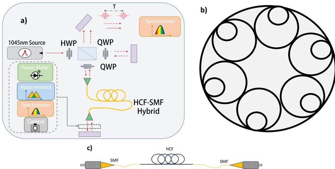
Figure 2: a) Michelson interferometer setup to characterise the >50m hybrid cable. b) 'Revolver' design of typical nested anti resonant nodeless hollow core fibre. c) Hybrid cable design, HCF terminated by two SMF pigtailed of differing length that cancel the dispersion in the 50m of HCF
