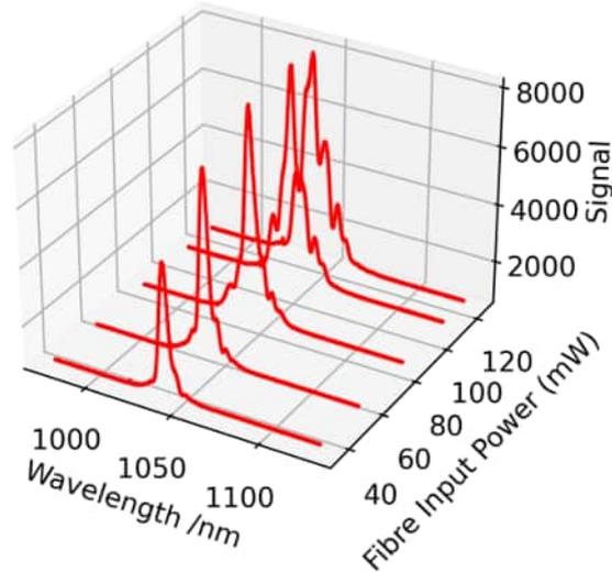
Figure 5: Evolution of the spectral envelope of the light with increasing power coupling into the fibre.
