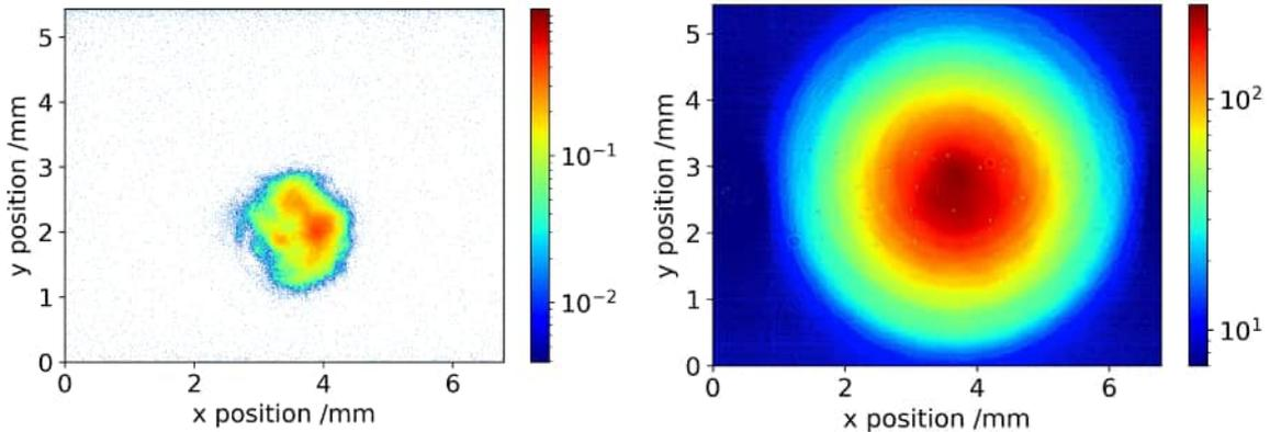
Figure 6: (Left) Spatial profile of the Insight DeepSee prior to the fibre input. (Right) Spatial profile at the output of the fibre. Image colour scales are arbitrary.
