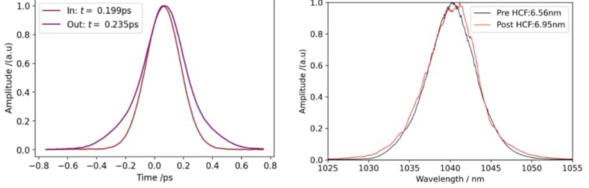
Figure 3: Measurements of the pulses autocorrelation and spectrum after a single pass of the 50m fibre.
