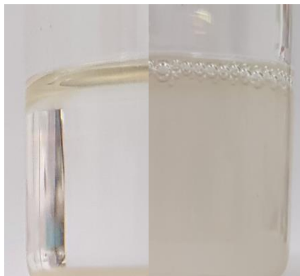
Figure 3 - An example of the changes of dispersion stability before (left) and after (right) silanization treatment of the particles [in Brij 40, after 3h]
