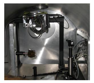
Figure 3. The new G1 mount in place in the chamber, without the grating. The antenna for RF cleaning can be seen in front of the mount. The back mirror and its mount fit on the back of the breadboard behind the black frame.
