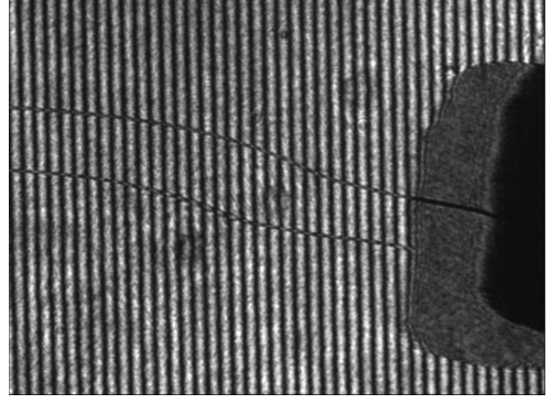
Figure 5: Interferometry image of a 25 micron horizontal wire at focus to simulate a plasma channel.
