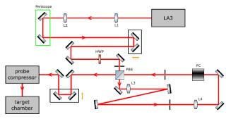
Figure 1: Diagram of the experimental setup. L1: f = 3 m; L2: f = 2 m; L3: f = 1 m; L4: f = 1 m; HWP: Half-wave plate; PBS: Polarising beamsplitter; PC: Pockels cell (Gooch & Housego TX 7595)
