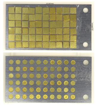
Figure 5: (top) Upper side of target array with sixty 2.8 mm square gold foil targets that are 30 µm thick; (bottom): Laserfacing side of (same) target array
