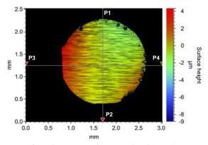
Figure 6: Foil position and topography of a single aperture in an assembled target array (from laser-facing side)
