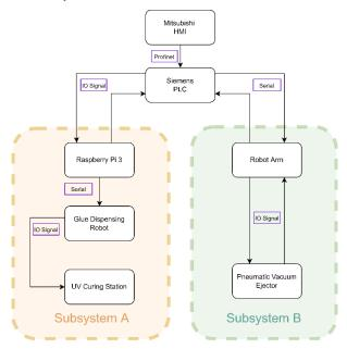
Figure 2: Communication System Architecture Diagram
