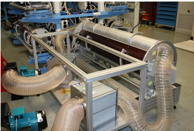
Figure 10. Photograph of the prototype amplifier in place for testing in the Vulcan amplifier.
