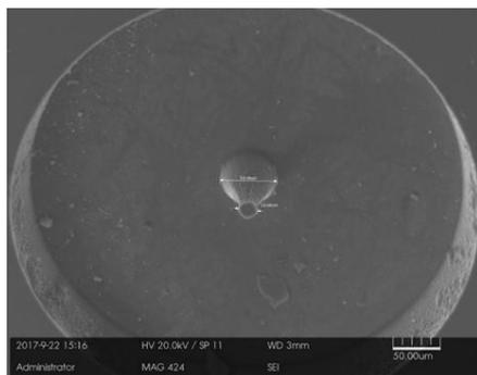
Fig. 1 – TEM image of Si conical target (courtesy of CLF target fabrication group and Scitech precision)
