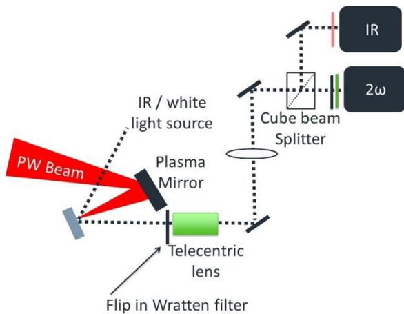
**Fig. 2 – In-situ layout of the alignment system**
