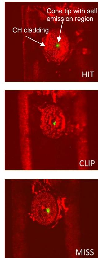
**Fig. 3 – a) image of self-emission directly on cone tip, b) clipping the cone tip, and c) completely displaced from the cone tip**
