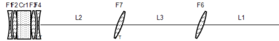
Figure 4: Arrangement of ring cavity, with astigmatic thermal lens on the YLF rod, one spherical and one cylindrical lens.
