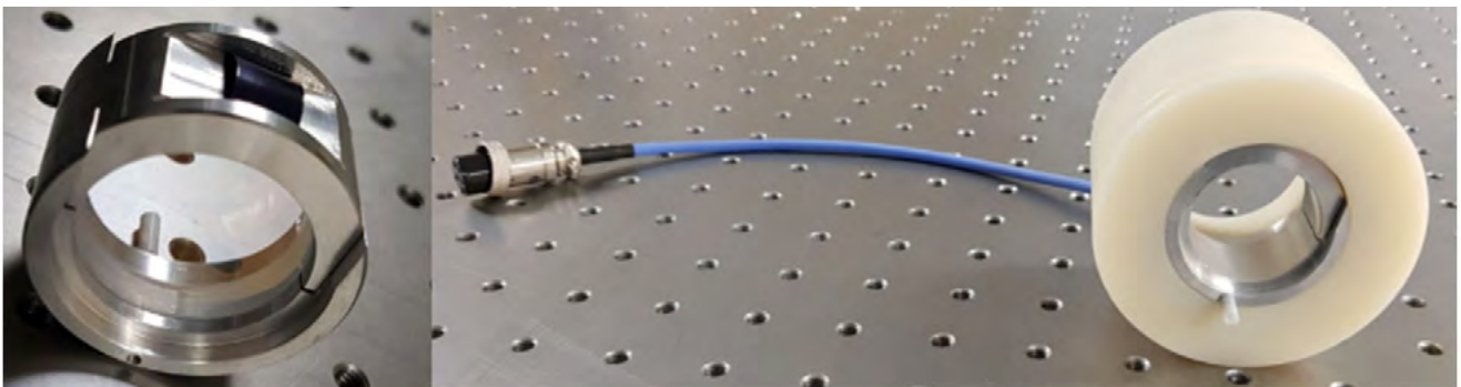
Photographs of LBO crystal oven components. The photo on the left shows the spring-loaded metallic crystal holder with the crystal in place. This is placed inside the oven unit (the photo on the right). The oven is then connected to a separate temperature control unit.
