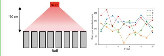
Rail calibration schematic (left) and results (right) demonstrating high variability in uniform set of crystals. Subtle variation in average reflective coefficient can explain the measured variation in yield.
