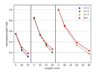
Light yield from a scintillator as a function of cross-section and aspect ratio, comparing the results from Cherry et al.<sup>[1]</sup> with the presented Monte Carlo simulation
