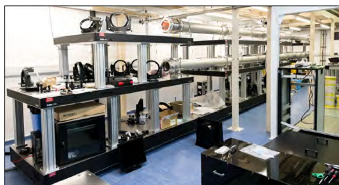
Figure 2: Three-tier table installed in LA4. A large-aperture (90 mm) LBO OPA stage on the bottom level will be pumped by a frequency-converted Vulcan long pulse beam, delivered from the top level.
