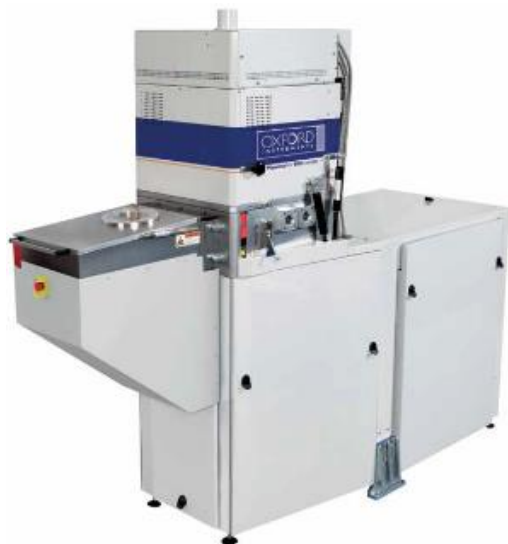
Figure 3: The CLF Deep Reactive Ion etching system
