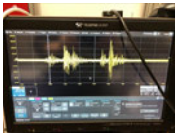
Figure 2: EMP noise generated by the two capacitor banks in the area in which the data acquisition device operates can interfere with the trigger.
