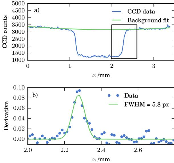
Figure 3: a) Averaged lineout through most opaque filter element, and fitted 2<sup>nd</sup>-order polynomial background. b) Derivative of ESF highlighted in a), with best-fit Gaussian overlaid.
