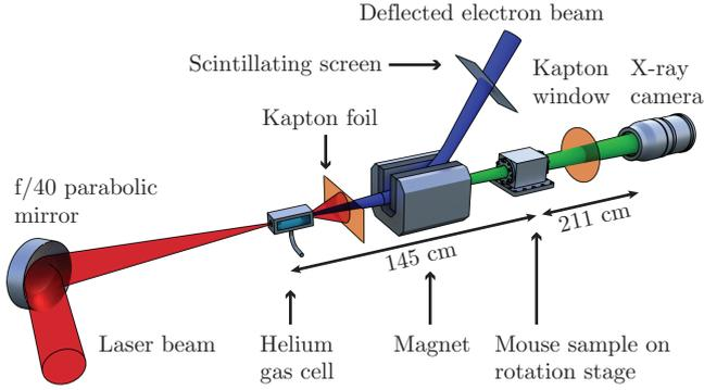
Figure 1: The x-ray beamline layout inside the main Gemini vacuum chamber. One of the Gemini beams (red) is focussed into a helium gas cell, producing co-propagating electron (blue) and x-ray (green) beams.
