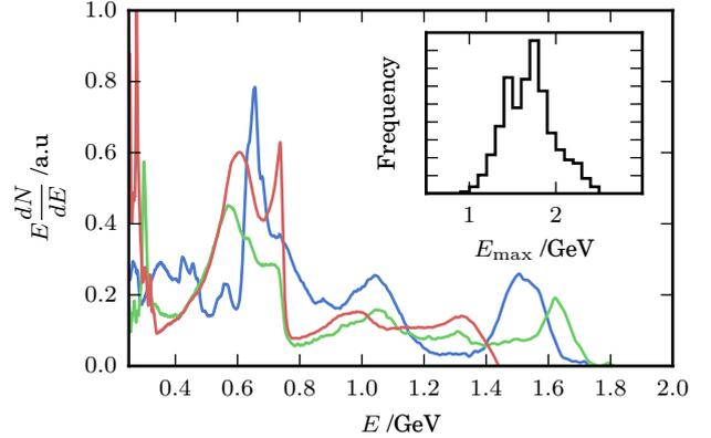
Figure 2: Typical electron spectra as recorded during the imaging shots, consisting of high-charge,  $\sim 0.7 \text{ GeV}$  and low-charge,  $\sim 1.5 \text{ GeV}$  components. *Inset* - histogram of peak electron energies during imaging shots.
