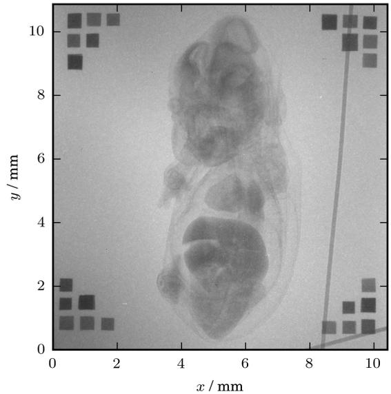
Figure 4: An exemplary radiograph of the mouse sample. The axes refer to spatial dimensions at the object plane. The squares in each corner are elemental filters for the on-shot transmission spectroscopy, and the thin wires act as fiducials to account for the source motion.
