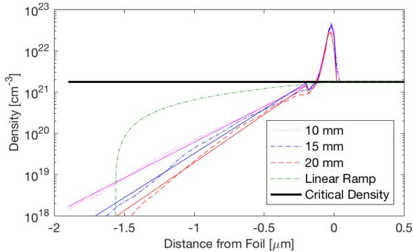
Figure 2: Electron density distribution resulting from the interaction between the pedestal of the laser pulse and the Kapton tape from the FLASH simulations and their exponential fits. The critical density is marked in black.
