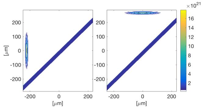
Figure 3: Left: Start of the simulation, the laser pulse coming from the left side of the window in 45° degrees towards the tape. Right: End of the simulation at which the laser pulse was reflected on the foil (in blue here).
