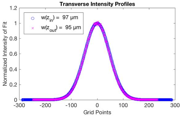
Figure 5: Transverse profile of the incoming and reflected s-polarised pulse for the plasma mirror being 15 mm in front of the focal plane.
