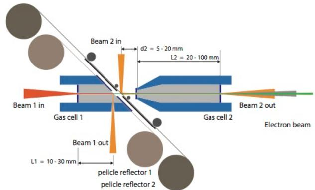
Figure 1: Possible set-up of a Laser Plasma-Wakefield staging experiment. A first laser beam is injected into a gas cell creating an accelerated electron bunch. A plasma mirror on a tape drive extracts the beam and a second tape drive injects a second laser pulse into a second gas cell to accelerate the electron beam even further.
