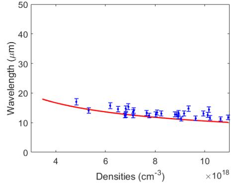
**Figure 4.** Plot of wakefield wavelengths against the plasma densities. The red line shows the theoretical wavelength.
