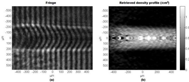
**Figure 2.** Mach-Zehnder interferometer result on the plasma density profile diagnostic. The modulation at the axis position in Figure (b) is due to the singularity near the axis in Abel inversion.
