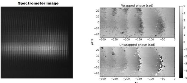
**Figure 3.** (Left) The spectrometer image of the spectral interferometry by the oblique angle probe pulses. (Right) The retrieved wrapped and unwrapped phase modulation when the plasma was present.
