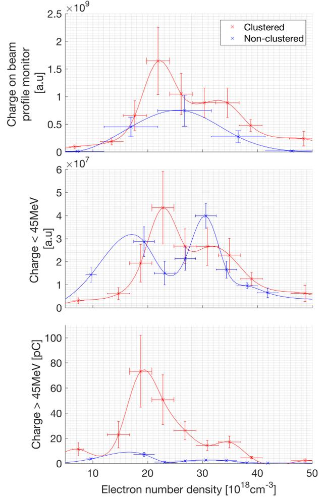
Figure 6: Comparison of beam charge between the clustered (red) & non-clustered (blue) on a) Beam profile monitor, b) Low energy electron spectrometer and c) High energy electron spectrometer.
