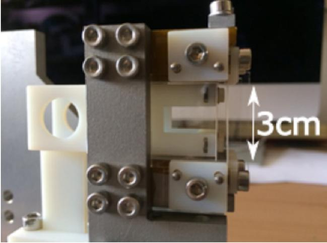
Figure 4: Gas cell used in this experiment
