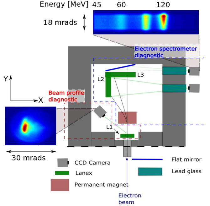
Figure 3: Particle diagnostics layout
