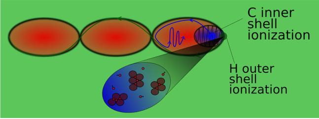
Figure 1: Blue path represents the path taken by electrons which are injected by cluster enhanced ionisation injection.
