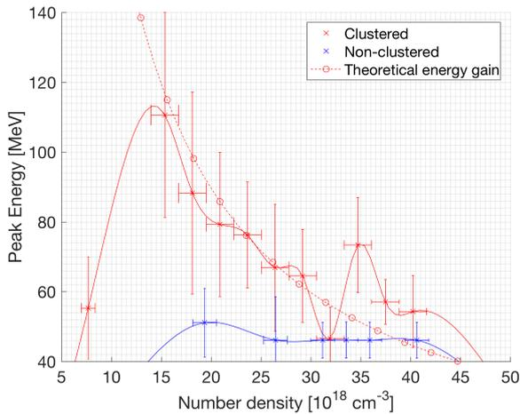
Figure 5: Peak electron energy. The linear 1D energy gain is given by  $W_{\max}[\text{eV}] = \frac{2m_e c^2 n_e}{n_e}$
