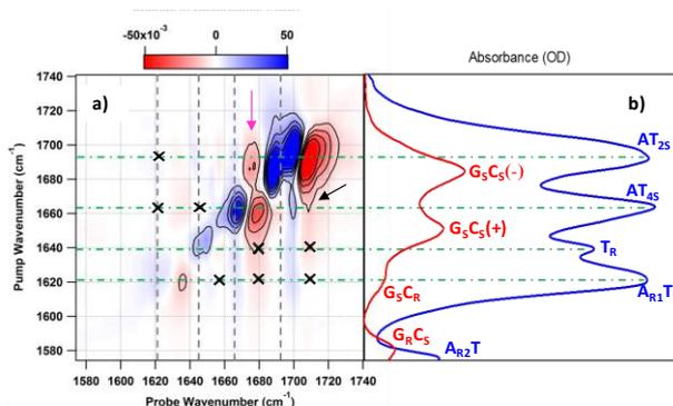
**Figure 2.** a) 2D-IR difference spectrum arising from the binding of Hoechst33258 to a 10-mer dsDNA oligomer featuring the AAATTT motif. Crosses show locations of small off-diagonal features. b) FTIR spectra of GC and AT-only DNA sequences show that the perturbation of the DNA spectrum occurs exclusively within the AT region of the dsDNA molecule.<sup>2</sup>
