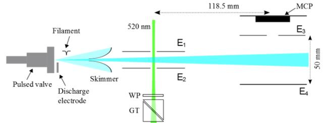
**Figure 1:** Experimental setup. The light from the pulsed dye laser is incident upon a supersonic beam of helium atoms in the metastable  $1s2s\ 2^3S_1$  state. By scanning the wavelength between 520 nm and 524 nm two-photon transitions are driven to Rydberg states in the range from  $n = 20$  up to the ionization limit. The Rydberg atoms are detected by pulsed field ionization in a field of strength 800 V/cm between electrodes E3 and E4.
