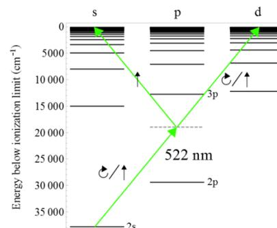
**Figure 2:** Energy level diagram of helium, showing the possible excitation channels for the two-photon transition, depending on the laser light polarization.
