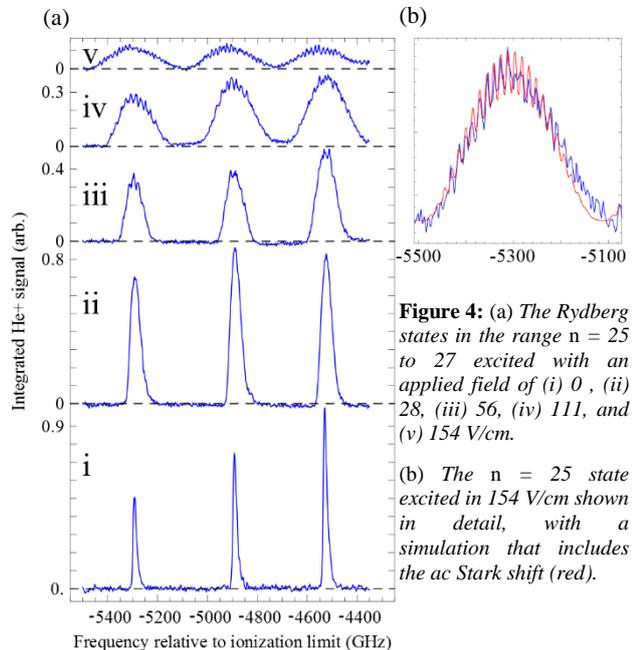
**Figure 4:** (a) The Rydberg states in the range  $n = 25$  to  $27$  excited with an applied field of (i)  $0$ , (ii)  $28$ , (iii)  $56$ , (iv)  $111$ , and (v)  $154$  V/cm. (b) The  $n = 25$  state excited in  $154$  V/cm shown in detail, with a simulation that includes the ac Stark shift (red).
