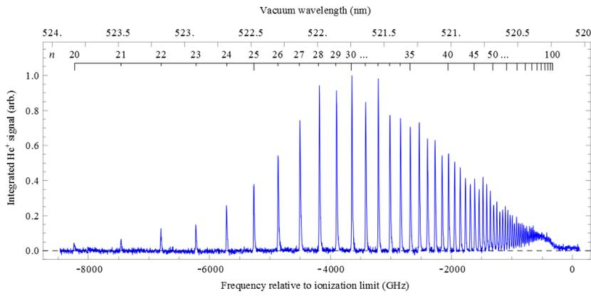
**Figure 3:** Recorded spectrum of  $|m|=2$  Rydberg states of helium, populated by non-resonant two-photon excitation using circularly polarized light. Rydberg states in the range  $20 \leq n < 100$  are efficiently populated, with states up to  $n = 76$  clearly resolved.
