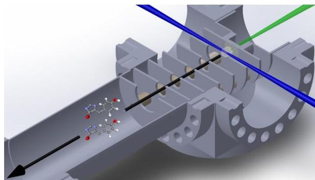
**Figure 1:** The experimental interaction region. The solid sample is placed on a thin foil (10  $\mu$ m) which is irradiated with a desorption laser on the reverse side. The resulting plume is ionised by a femtosecond laser and the ions extracted into a time of flight mass spectrometer.
