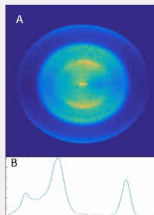
Photoelectron image (A) and spectrum (B) of CS<sub>2</sub> following excitation with UV (6.2 eV) and probing with XUV (15.5 eV) light.
