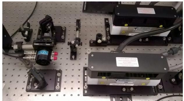
Figure 3. Pulse shaping Pockels cell
