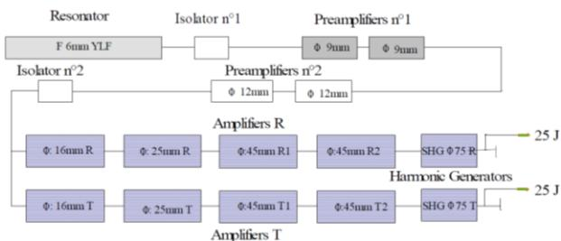
Figure 1. Quantel laser configuration
