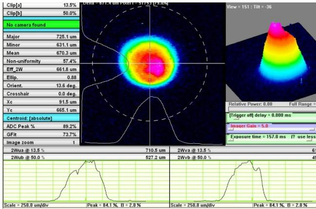
Figure 4. Quantel beam full energy focal spot
