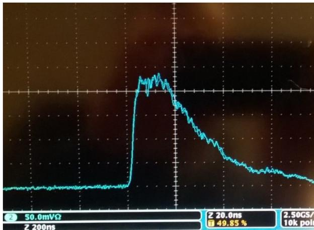
Figure 5. Temporal profile of a full energy shaped Quantel pulse
