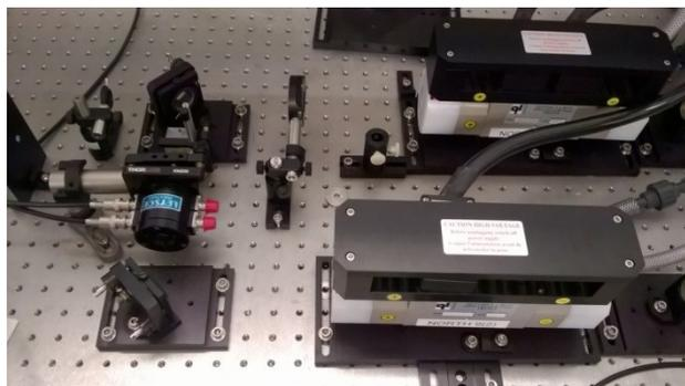
Figure 3. Pulse shaping Pockels cell
