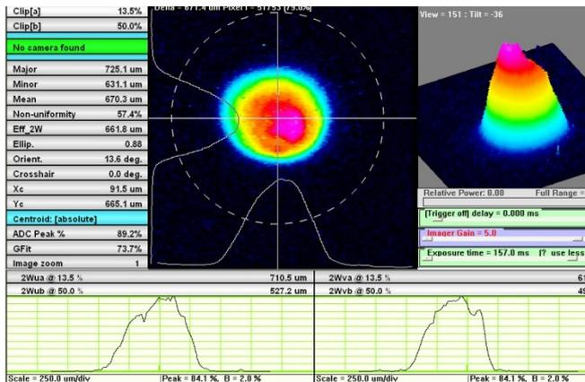
Figure 4. Quantel beam full energy focal spot
