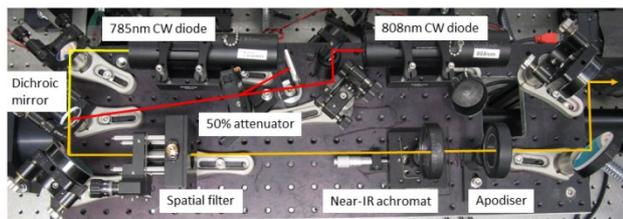
Figure 1. Photograph showing the layout of the dual wavelength CW diodes in the Gemini front end room, with beam lines indicated.
