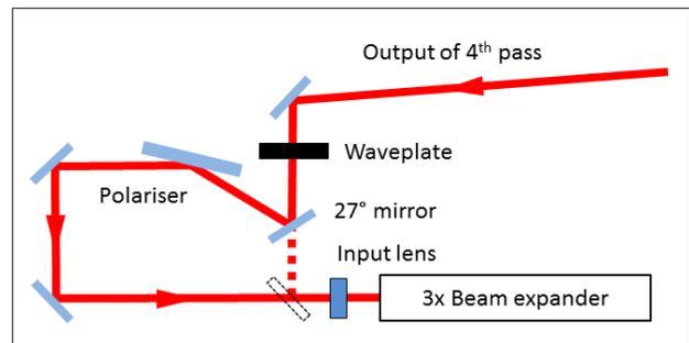
Figure 3. Output section of a Gemini amplifier showing the new (solid line) and old (dashed line) beam paths, and the integration of the energy-control waveplate and polariser.
