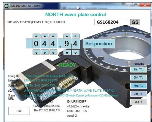
Figure 4. Screenshot of the waveplate control app, showing the controls for setting the stage position, and the buttons for the preset positions.
