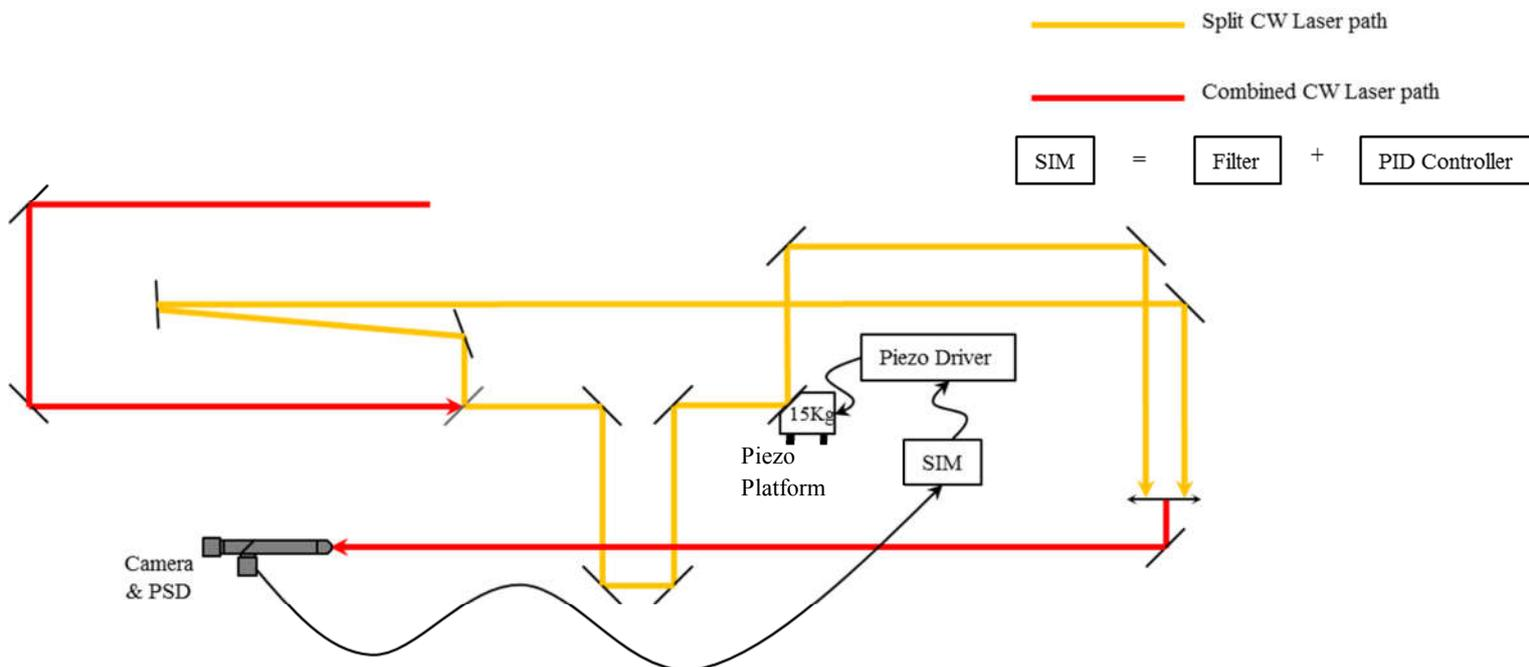
**Fig. 2:** Schematic setup of the HAPPIE Lab setup used to achieve fast beam stabilisation.
