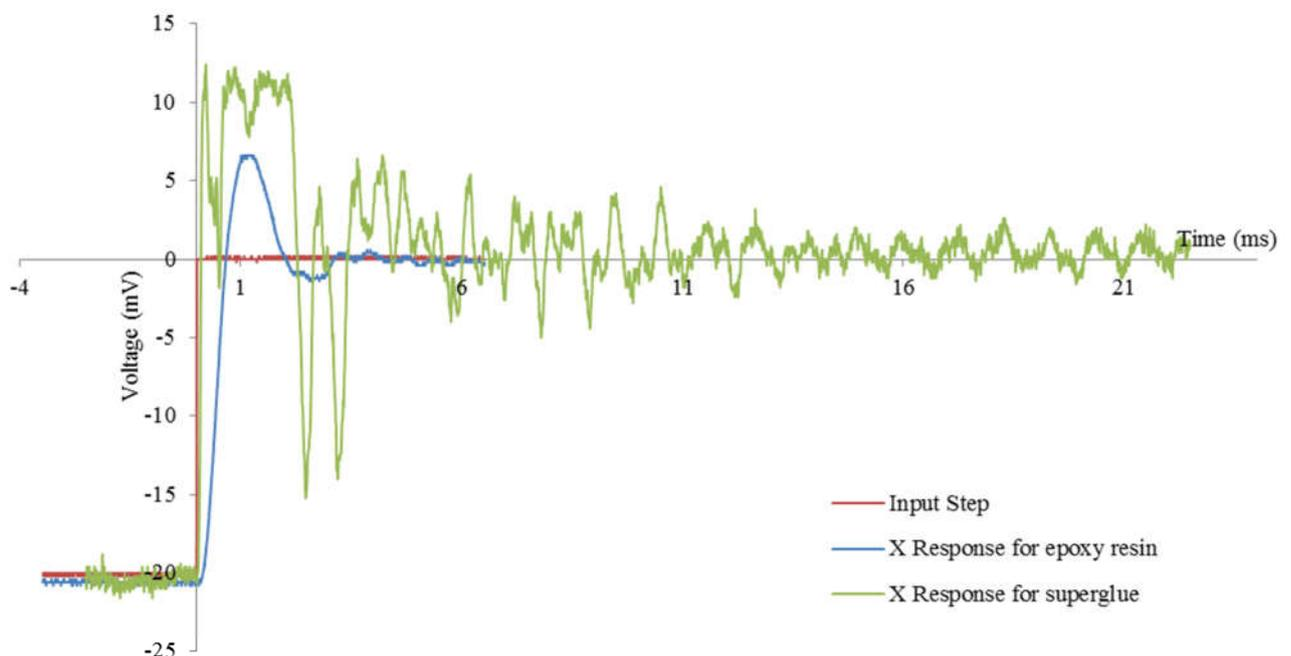
**Fig. 6:** Response within the X axis of two mirrors when exposed to a square input signal.
