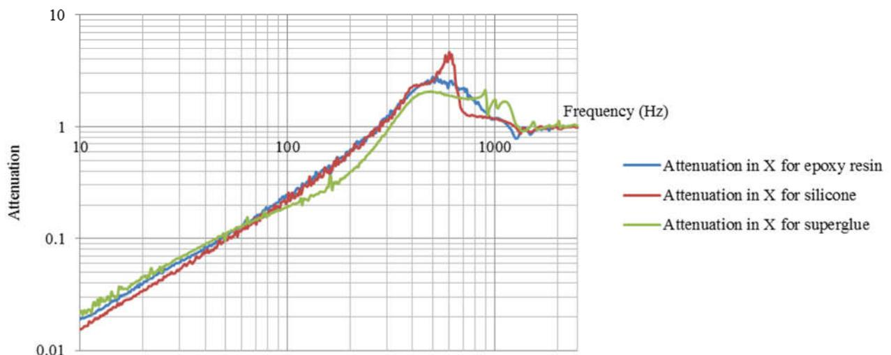
**Fig. 4:** Attenuation of the far field's vibrations within the X axis for each different mirror across a range of frequencies from 10 Hz up to 2500 Hz.
