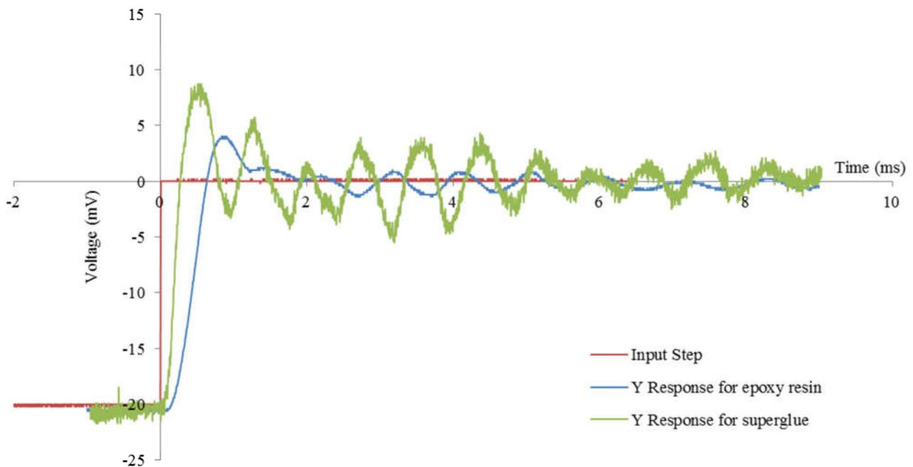
**Fig. 7:** Response within the Y axis of two mirrors when exposed to a square input signal.
