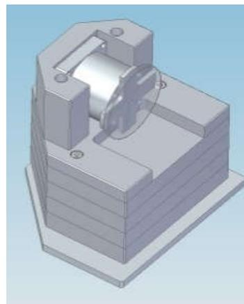
**Fig. 1:** Vibration damping mount system for the piezo driver and mirror. The mount weighs approximately 15 kg in order to optimise the range of frequencies which the Sorbothane feet isolate.
