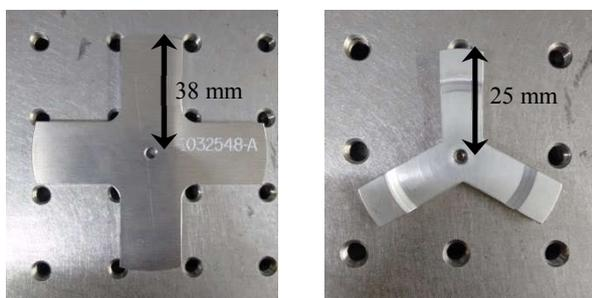
**Fig. 3:** Left – 4 point cross mounting adaptor.
