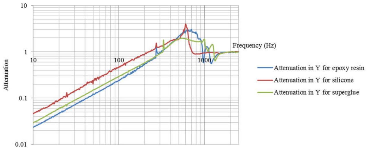
**Fig. 5:** Attenuation of the far field's vibrations within the Y axis for each different mirror across a range of frequencies from 10 Hz up to 2500 Hz.
