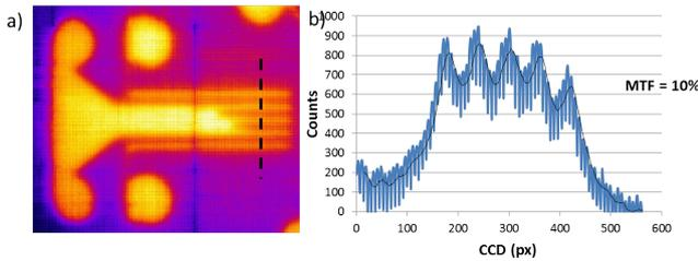
**Figure(3)** a) shows a high magnification radiograph from the high energy phantom, b) is the corresponding line out across the 200μm slits shown and an MTF when of the background subtracted image. Features are clearly visible with an modulation transfer function (MTF) of 10% indicating that the source must have been smaller than 200μm.
