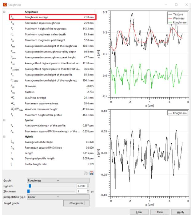
Figure 3: shows the roughness tool in Gwyddion. In the red box is the average one-dimensional roughness.
