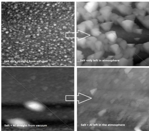
Figure 5: Image showing a comparison of a coating straight from the vacuum vs being left in the atmosphere. (Note that the image 'from vacuum' and 'left in atmosphere' are not the same area).
