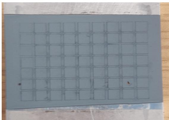
Figure 1 showing a thin film coating of Al on an array of targets.
