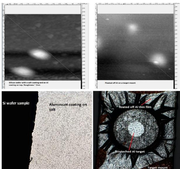
Figure 6: Image showing an AFM scan of the floated off Al
