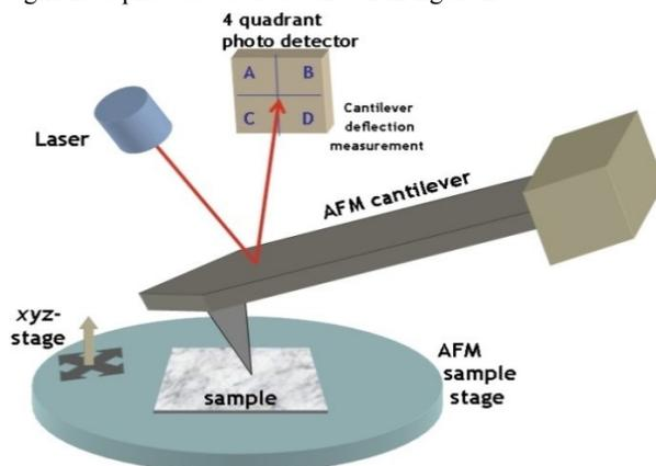
Figure 2 showing an AFM in action<sup>4</sup>.
