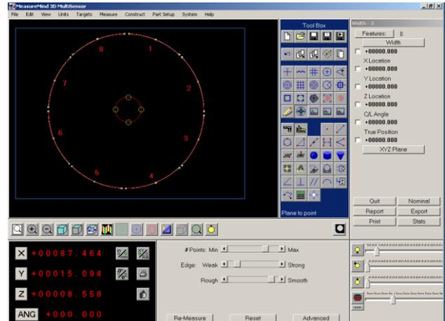
Figure 5. CMM characterisation of the target wheel and wafer segments. Green lines indicate measured features and red lines indicate constructed features inferred from measurements.
