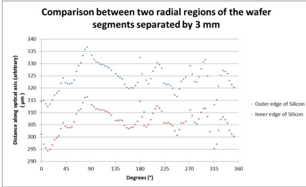
Figure 7. Chromatic confocal displacement results across two radial regions of the target wafer segments showing the change in z position over 360°.
