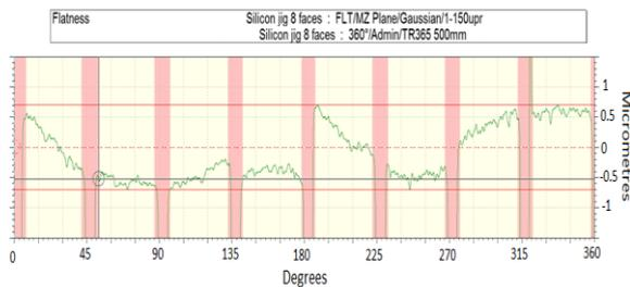
Figure 4. Surface metrology of the ceramic interface wheel over each of the eight target segment mounting slots.
