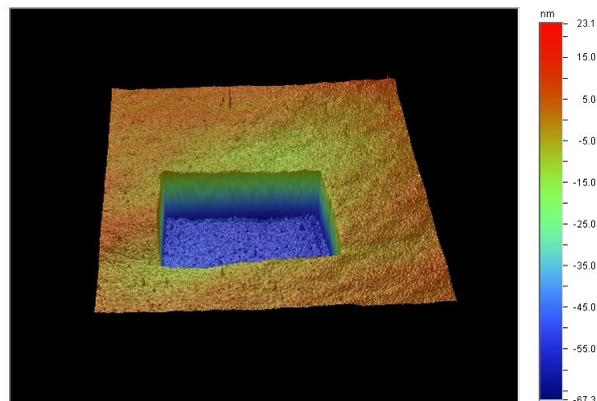
Figure 2. 3D white light interferometric topography of  $\text{Si}_3\text{N}_4$  surface across 350  $\mu\text{m}$  square target aperture.
