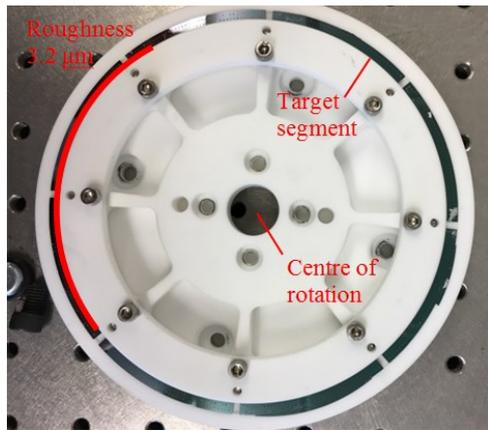
Figure 3. Interface wheel mounted with target segments.
