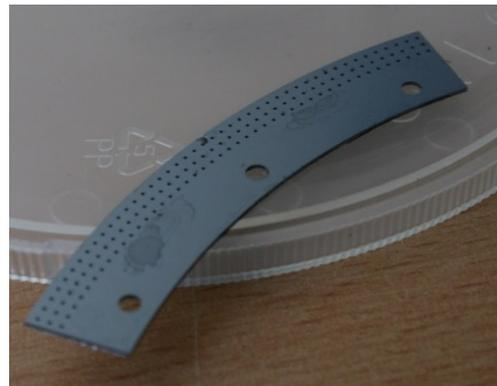
Figure 1. Etched HAMS silicon wafer segment with three rows of 100nm thick  $\text{Si}_3\text{N}_4$  target apertures each comprising 44 targets.
