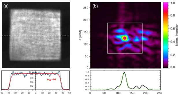
**Figure 14:** (a) Near-field and (b) far-field profiles of DiPOLE100 output beam measured at 102 J and 10 Hz.
