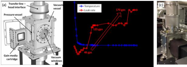
**Figure 9:** (a) 3D model, (b) helium leak rate dependence on MFR at 150 K, and (c) photograph of installed 100J cryo-amplifier head at HiLASE.
