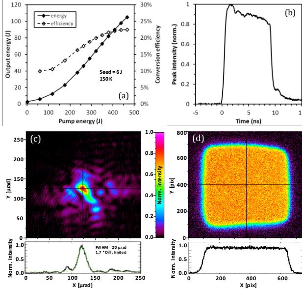
Figure 2: (a) Energy conversion; (b) temporal profile measured with 4 GHz bandwidth limit; (c) far-field intensity image and (d) spatial uniformity profile of output beam with cross-section profiles from DiPOLE100 operating at 10 Hz.
