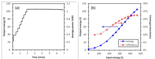
**Figure 12:** (a) Output energy ramp to 105 J and (b) energy and conversion efficiency when final cryo-amplifier operated to 1 kW average power level at 10 Hz at HiLASE.
