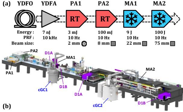
Figure 1: a) Schematic of DiPOLE100 amplifier chain showing typical output performance after each amplifier stage, including free-space beam size and shape: YDFO = Yb-silica fibre oscillator; YDFA = Yb-silica fibre amplifier (inc. temporal pulse shaping); PA = room-temperature pre-amplifier (1=Yb:CaF<sub>2</sub> regenerative, 2=Yb:YAG multi-pass); MA = main cryogenic amplifier (ceramic Yb:YAG multi-slab). (b) 3D model of DiPOLE100 system: D = Diode pumps; cGC = cryogenic gas coolers.
