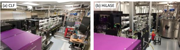
**Figure 10:** Photographs of 100J cryo-amplifier stage (a) prior to disassembly at the CLF and (b) after rebuild at HiLASE.
