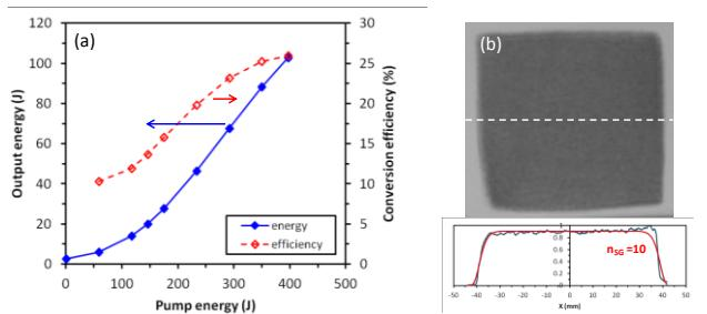
**Figure 11:** (a) Output energy and conversion efficiency, and (b) burn pattern captured at 103 J with cross-section when final cryo-amplifier operated at 1 Hz at HiLASE.
