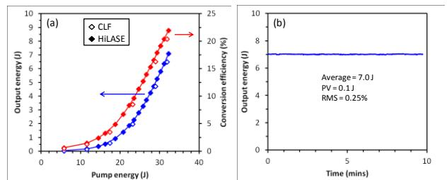
**Figure 8:** (a) Output energy and conversion efficiency (hollow and solid diamonds represent data measured at the CLF and HiLASE, respectively), and (b) short-term energy stability of the 10J cryo-preamplifier output at 10 Hz.
