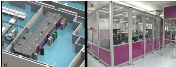
**Figure 6:** (a) 3D model of DiPOLE100 enclosure and (b) photograph taken from the 100J cryo-amplifier end of system at HiLASE.
