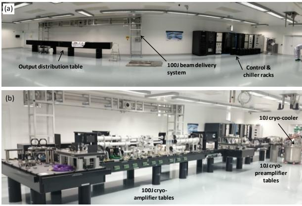
**Figure 5:** Photographs of the HiLASE laboratory (a) before and (b) after optical table assembly.
