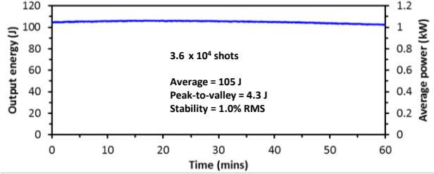
Figure 3: Long term energy stability over 1 hour at 10 Hz.
