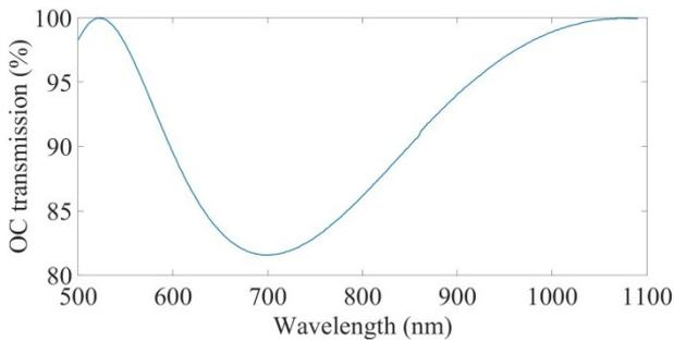
Fig. 2 - Output coupler transmission profile
