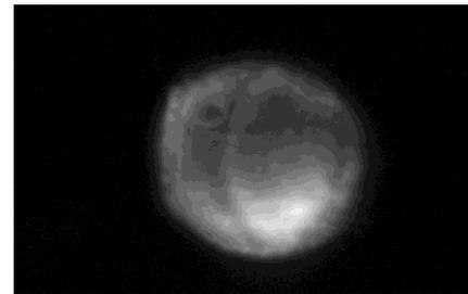
Fig. 5 – Characteristic OPA near field profile
