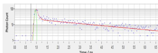
Figure 1: Typical photon decay curve obtained when performing FLIM in this study. The short sharp peak at early time points is characteristic of surface plasmon resonance from the AuNP and the long, slow tail off afterwards due to fluorescence from cellular material.
