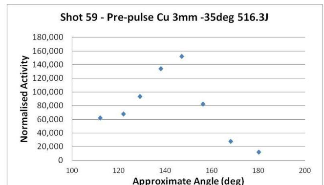
**Figure 5: The result from a 3mm copper target.**
