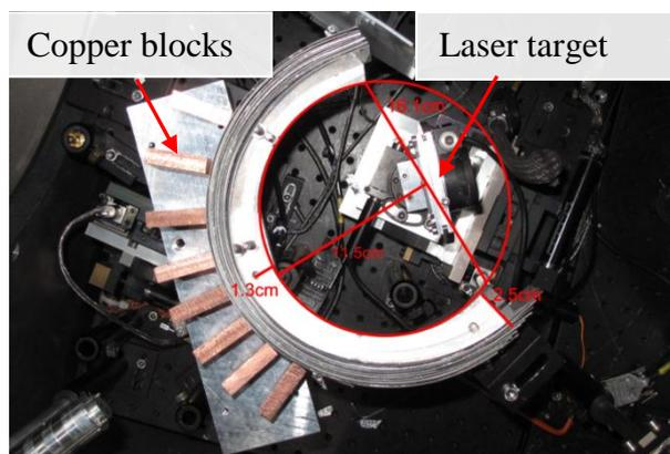
Figure 2: A curved array of eight copper blocks inside the chamber and around the laser target.
