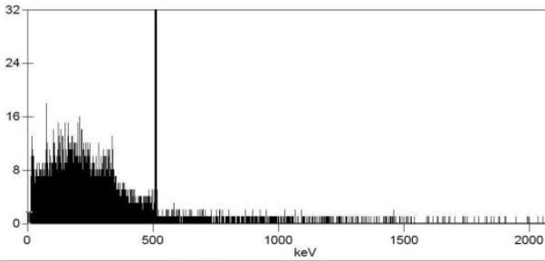
**Figure 3: A HP:Ge detector reading of a copper block showing the 511keV activation line.**
