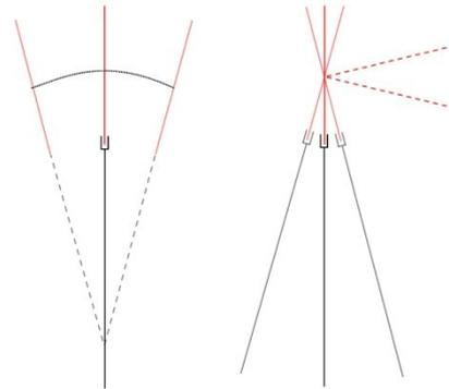
**Figure 3. A schematic illustrating how the target (in red) translates in z if the axis of rotation is not through the focus of the lens. If the axis of rotation is through the centre of the target, as on the right, the target does not translate in z. The target is viewed side-on.**
