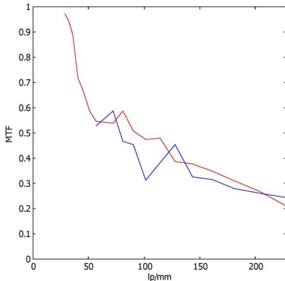
**Figure 2. The Modulation Transfer Function for the Firefly System (red) and the Mitutoyo System (blue). Both systems perform similarly in the region of 80-230 lp/mm.**
