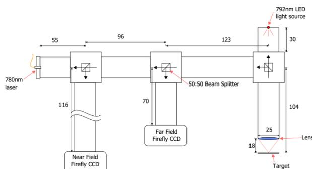
**Figure 1. A schematic of the Firefly system. All beam splitters are 50:50. The LED on the top right emits at  $792\pm 30\text{nm}$  and is used to illuminate the target. The laser, attached using an SMA fibre optic cable, is capable of giving information about the pointing of the target. All distances are in mm.**
