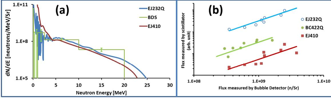
Figure 2: (a) Calibrated neutron spectra obtained from EJ232Q and EJ410 detectors compared with spectrum obtained by BDS in the same shot. (b) Comparison between neutron flux obtained from different scintillator detectors and the BDS for neutron energy in the range 2.5-20 MeV. The graph plots the comparison for three different scintillator detectors, EJ232Q, BC422Q and EJ410, obtained over a number of shots. The solid lines show linear fits to the data points.
