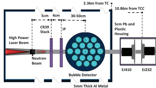
Figure 1: Schematic of experimental setup. The neutron beam generated by the laser-target interaction propagates through various diagnostics before reaching the scintillator detectors placed outside the interaction chamber.
