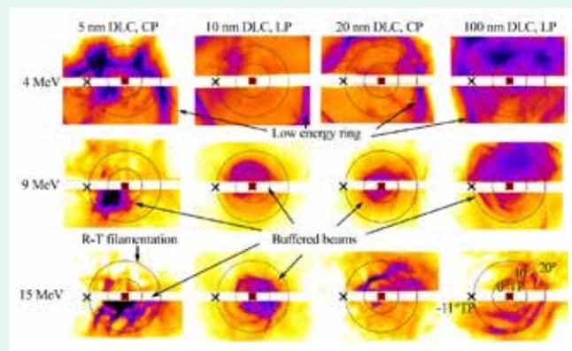
Selected radiochromic film layers from stack diagnostic showing proton beam pattern at different energy bands for different target thicknesses. The low energy beam (top row) is dominated by an annular ring, whereas at high energy (middle/bottom row) a collimated beam appears along the laser axis.
