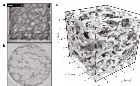
Tomographic reconstruction of trabecular bone sample: a, A raw image of the bone sample recorded on the x-ray camera. b, 2D reconstruction of a one-pixel high horizontal slice of the sample at the position indicated in a). c, Stacking together 1300 such slices generates a 3D voxel map of the bone sample. An isosurface marking the detailed structure of the bone surface is constructed, rendered using a ray-tracing method.
