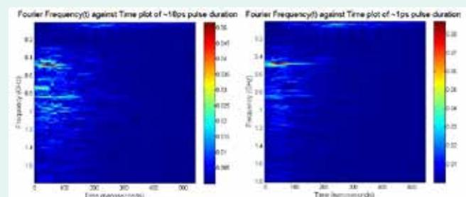
Comparison of the 1 ps pulse (Right) and the 18ps pulse (Left) using a Nyquist Fourier Transform Program
