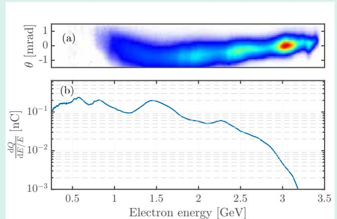
High-energy electron beam measured with the f/40 focusing geometry. Panel (a) shows the raw data, highlighting the beam's very narrow (~1 mrad) divergence. The electron beam spectrum is plotted in Panel (b), emphasizing the multi-GeV energy scale acceleration.
