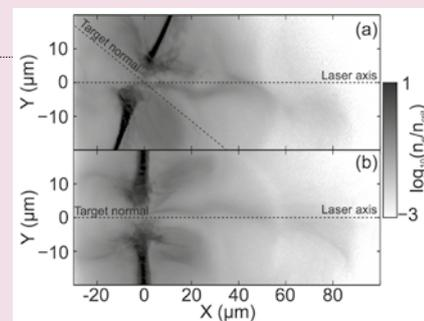
*2D Simulation results showing electron density for a target initialised at (a) 0° and (b) 30° incident angle to the laser at an example time of 0.3 ps after the peak of the laser pulse has reached the target surface.*
