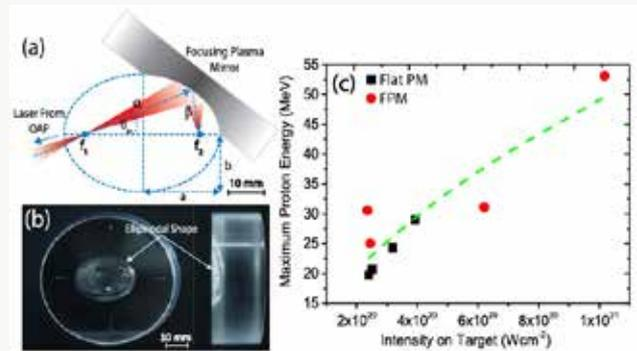
(a) Illustration of ellipsoidal focusing plasma mirror (FPM) concept. (b) Image of the manufactured FPM. (c) Plot of the max. proton energy achieved using either a FPM or flat PM.
