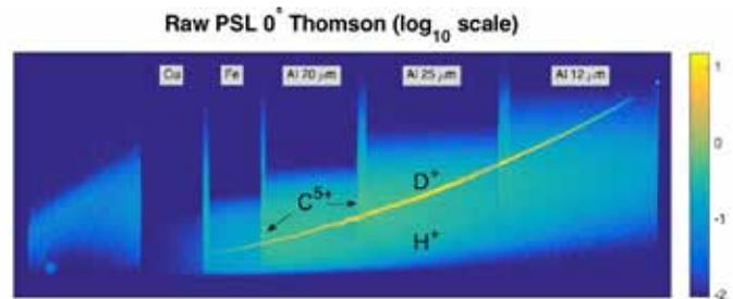
Raw Thomson parabola spectrometer data. The bright yellow line is the deuterium ion trace; a faint proton trace is also seen below; C ions are also present in the gaps of the heavy ion filters. The ratio of deuterium ions to protons is in excess of 99.9% demonstrating practically complete annihilation of the proton beam while achieving a bright deuterium ion beam.
