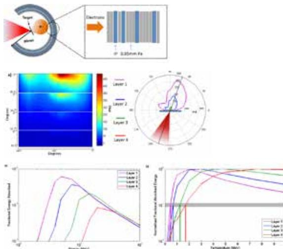
Top: Schematic of the diagnostic arrangement of Fuji BAS-TR Image Plate (IP) between 0.85mm Fe filter. Middle: The fractional absorption in the IP layers from mono-energetic electrons incident onto the array of Fe filters as a function of energy. Bottom: PSL signal from the remapped layers of IP between the Fe filtering from a 140J shot onto a  $100 \mu\text{m}$  Cu target and its corresponding polar plot.
