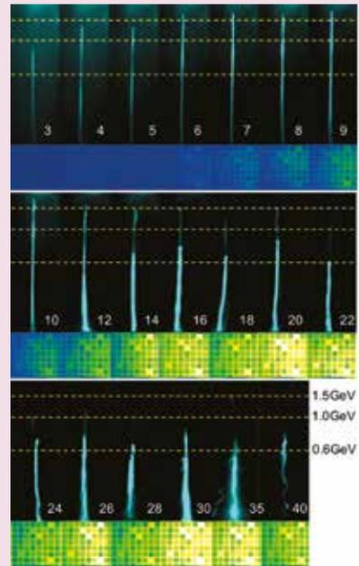
Top: Electron spectra (black/blue) and betatron x-ray images (green) from an accelerator length scan, with length in mm denoted by the white numbers. The electron beam is dispersed vertically by energy. At 12 mm length a high charge per MeV electron beam was injected, which was correlated with a large increase in x-ray flux.
