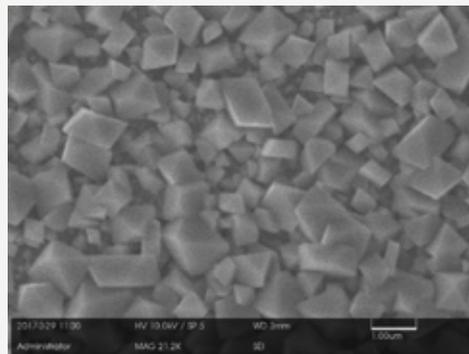
SEM image of copper surface formed on aluminium strip. Plating conditions: 18°C, 1 mol dm<sup>-3</sup> CuSO<sub>4</sub>, not stirred throughout plating time, 10mA applied.
