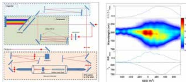
Left: Schematic of the experimental setup of the XPW generation system.
