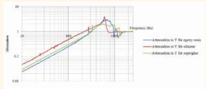
Attenuation of vibrations in the far field across a range of frequencies from 10 Hz up to 2500 Hz. Different adhesives for attaching the mirror substrate to the piezo platform produce varying responses.
