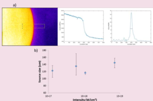
a) an example image cast by the penumbral aperture, with the two subsequent inset graphs being a lineout and the gradient showing the source size b) shows the results from the defocus scan on 100µm tantalum, error bars shown account for the asymmetry of the source and variance in the source further corrections can be made by accounting for the point spread function (PSF) of the filter layers.
