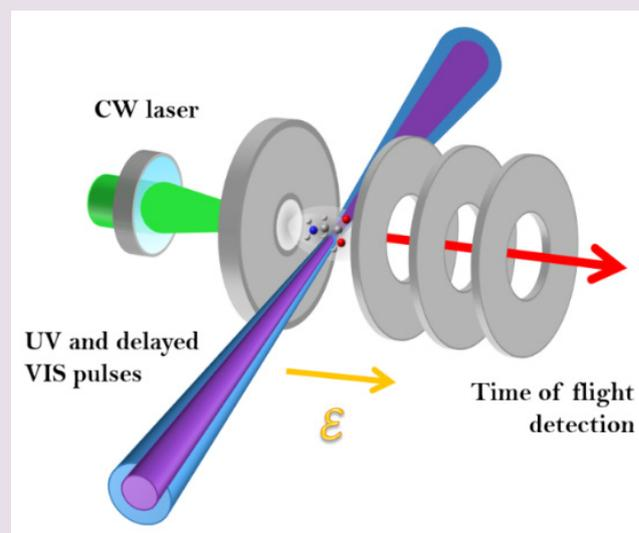
Schematic representation of the experiment. Femtosecond ultraviolet and visible laser pulses were focused into the interaction chamber, where they were absorbed by the molecules to form positive ions. By analysing the masses of the ions produced for different delays between the two laser pulses, the ultrafast dynamics were observed.
