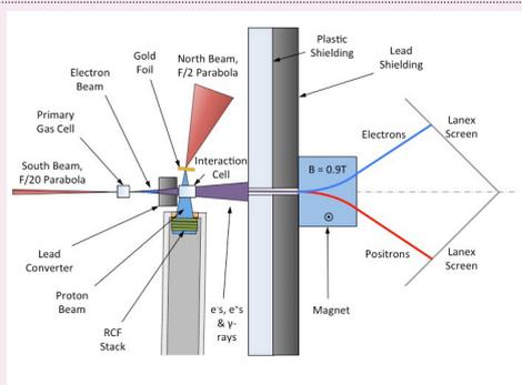
*Schematic of the experimental layout. Outside of the experimental plane, and not shown in the figure, is a collection optic used to image the rear surface of the interaction cell to observe the beam profile.*
