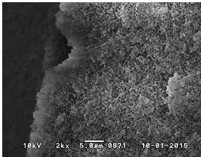
Top: 100mg/cc foam, Au coated, x2000 mag. Image used to characterise pore size used.
