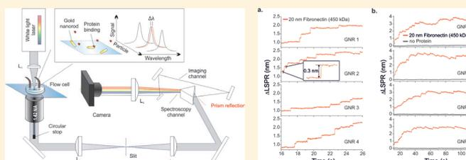
(Left): Experimental setup of the dark field microspectroscopy.
