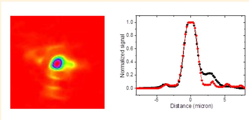
Focal spot of the pulsed beam using an adaptive optic and  $f/2$  parabola.
