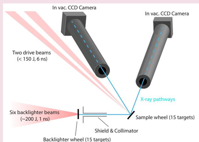
Experimental set-up within the target chamber.
