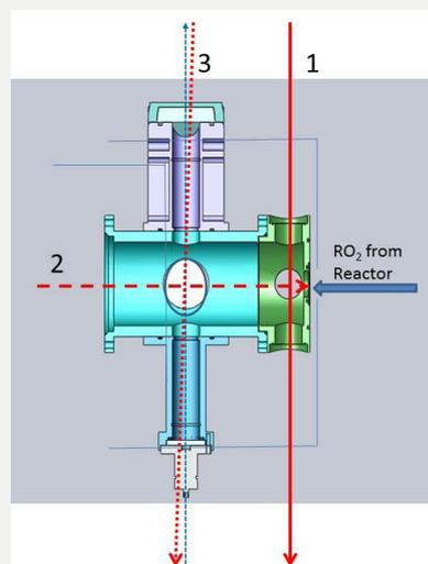
A solid model drawing of the photolysis cell. RO<sub>2</sub> radicals flow through the pinhole and are photolysed in the near UV with the NSL2 laser system using three geometries (in red), before OH is detected via the second laser (blue).
