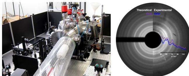
Left: The TRED apparatus at York. Right: Comparison between theoretical and experimental diffraction patterns and diffraction data, collected from a 20 nm-thick polycrystalline platinum sample.
