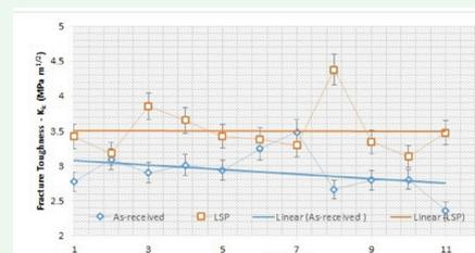
Surface hardness (top) and  $K_{Ic}$  (bottom) of the  $Si_3N_4$  advanced ceramic after LSP
