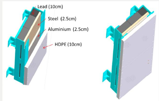
Engineering drawing of the frame that has been installed in Gemini TA3 to hold extra lead shielding vertically above the electron beamline.
