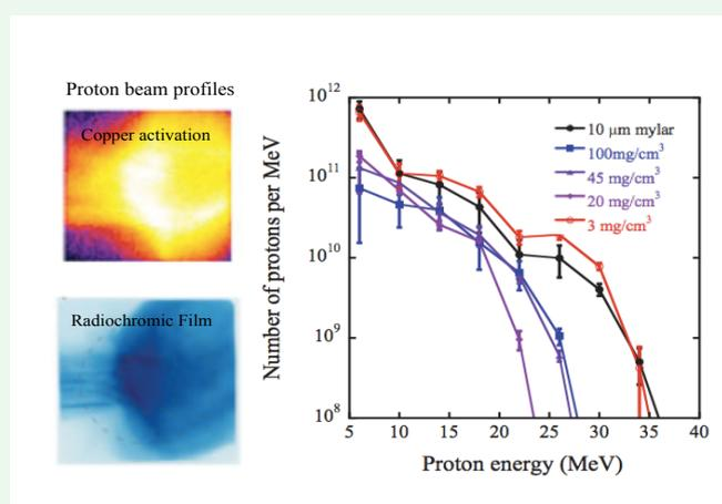
(Left) Proton beam profiles recorded using: (top) the copper activation stack and imaged post-shot using image plate detectors; and (bottom) directly on the radiochromic film stack layers for a 20 mg/cc foam target.
