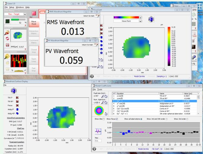
Screenshot from the AO control program, showing a well-corrected beam from Amplifier 3.
