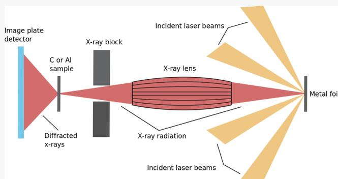
Top-down view of the experimental setup. The incident laser beams drive the He- $\alpha$  transition in the titanium foil on the right hand side of the diagram. The resulting line radiation is focused by the x-ray lens onto the target. The x-rays are diffracted according to Bragg's law and are detected by the image plate. The distance between the titanium target and the sample is 242.3 mm.
