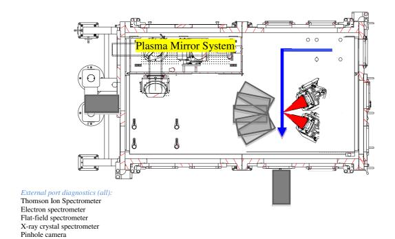
Raised level beam transport is shown below to aid planning of out of plane diagnostics.
