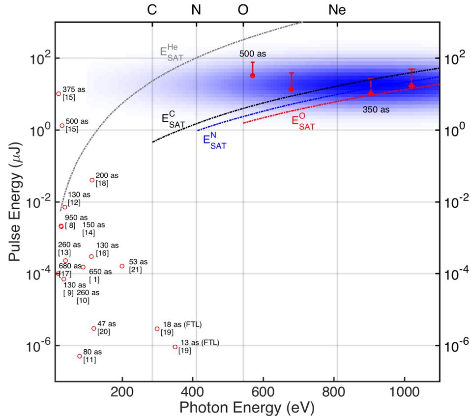
XLEAP intense enough to drive non-linear interactions across the SXR range. First evidence that it can drive electronic impulsive X-ray Raman recently seen.
