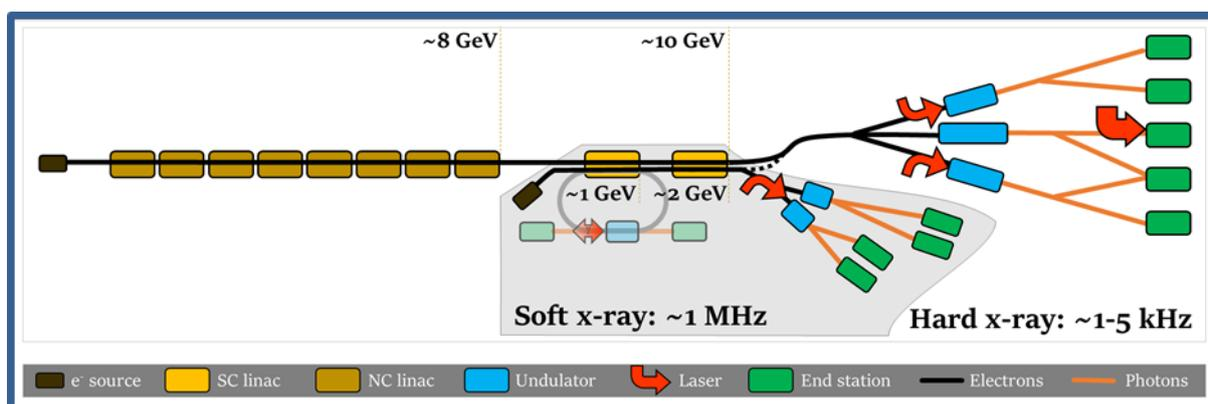
Figure 1.1: An outline design of one potential configuration with a unique combination of capabilities, able to deliver the science discussed in this case
