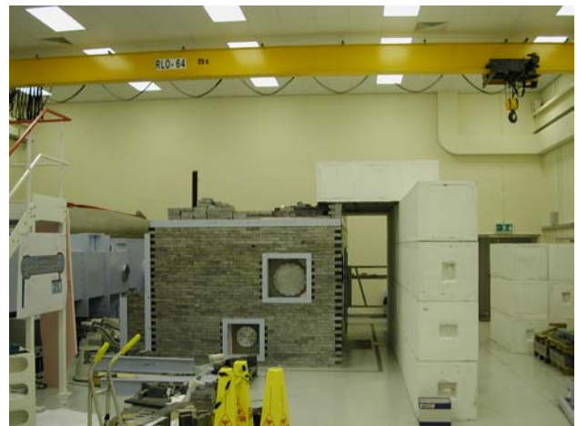
Figure 5. The concrete labyrinth for shielding the entrance of the interaction chamber.
