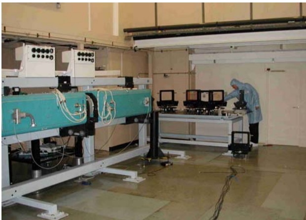
Figure 2. Photograph of LA4 during the commissioning phase, showing the last two 208 mm disc amplifiers and some of the turning mirrors. The final beam expansion optics are situated behind the temporary wall (at right).
