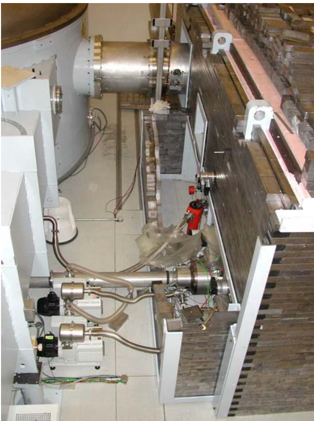
Figure 3. Lead housing for the vacuum system of the interaction chamber partially installed.
