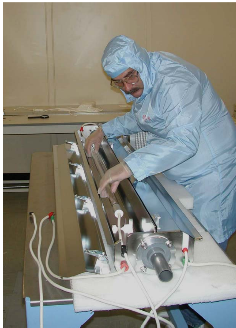
Figure 1. A flashlamp being loaded into the dual flashlamp tester by Andy Frackiewicz.
