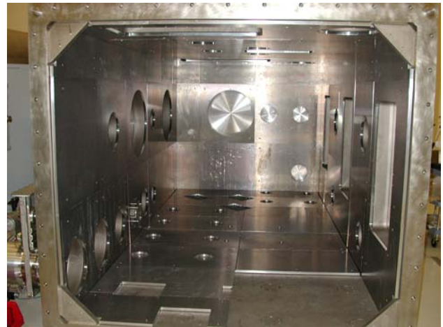
Figure 4. The interior of the interaction chamber with almost all of the Aluminium plates in place.
