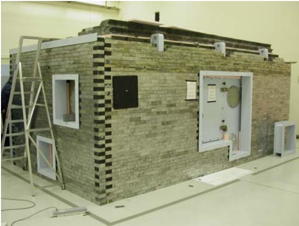
Figure 2. Lead shielding of the north and west walls of the interaction chamber. The two ports alongside the entrance door will be used as an optical port and a feedthrough port respectively. The lower port in the north wall is also a feedthrough port.
