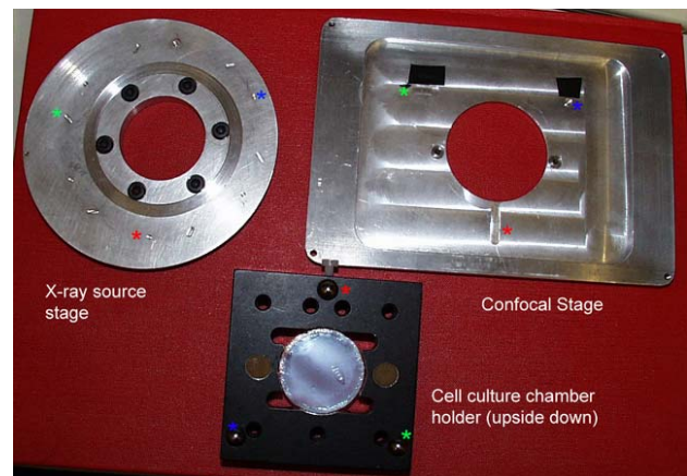
Figure 5. Images of the micropositioners from the x-ray source and the stage of the confocal microscope, and (upside down) the cell growth chamber holder. Coloured circles indicate triangulation points for one position of irradiation.
