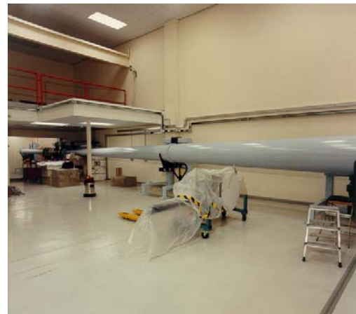
Photo 8. The vacuum spatial filter completed.
