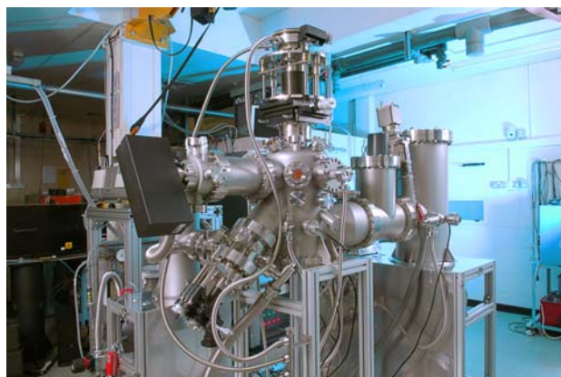
Figure 2. The UHV chamber in the Nanosecond science Laboratory (Lab B) at the Central Laser Facility.
