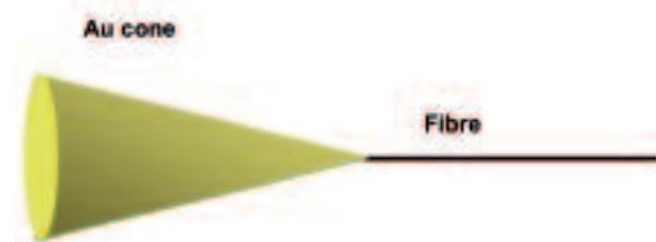
Figure 1. Typical cone –fibre target: The target consists of a Au re-entrant cone with 30^\circ open angle terminating in a flat 30 \mu\text{m} diameter disk, to which a CD fibre is attached.
