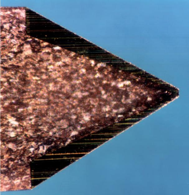
**Figure 4.** Sectioned and polished cone still on mandrel.
