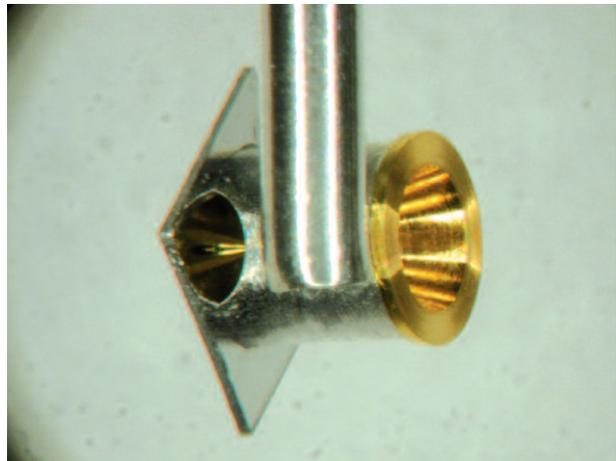
**Figure 6.** A fully assembled AFI target with stand off tube and foil package. The reflection of the cone tip can be seen in the foil.
