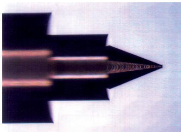
Figure 1. Copper mandrel with datum surfaces machined.
