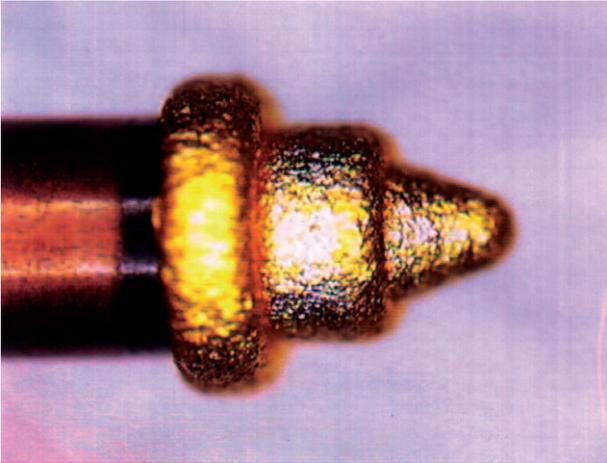
**Figure 3.** An electroplated part showing the gold deposit on the copper mandrel.
