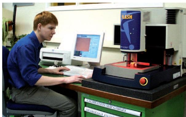
Figure 2. Inspection of a mandrel using on optical co-ordinate measuring machine.
