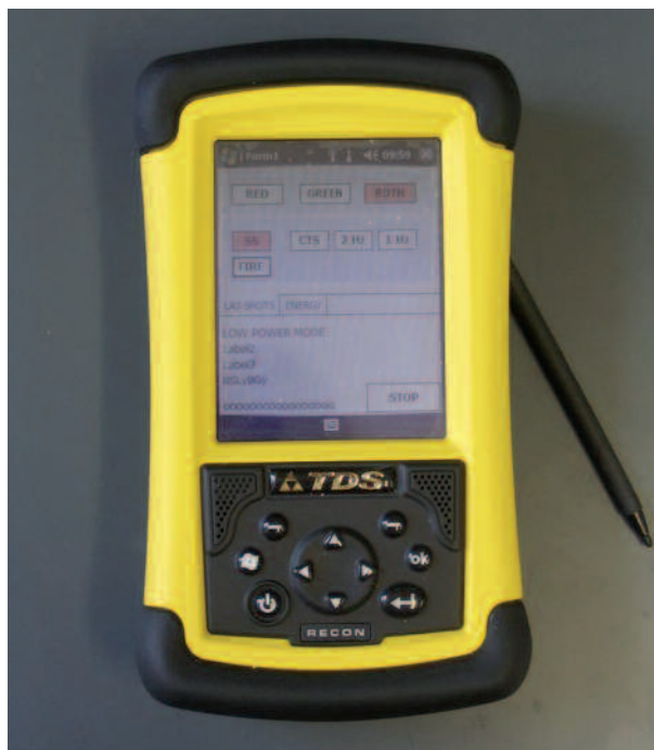
Figure 4. Picture of wireless pad used for shot control in Astra LA3.
