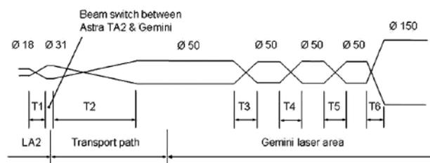
Figure 1. Schematic of the optical system that transports the beam from Astra to the Gemini pulse compressors.
