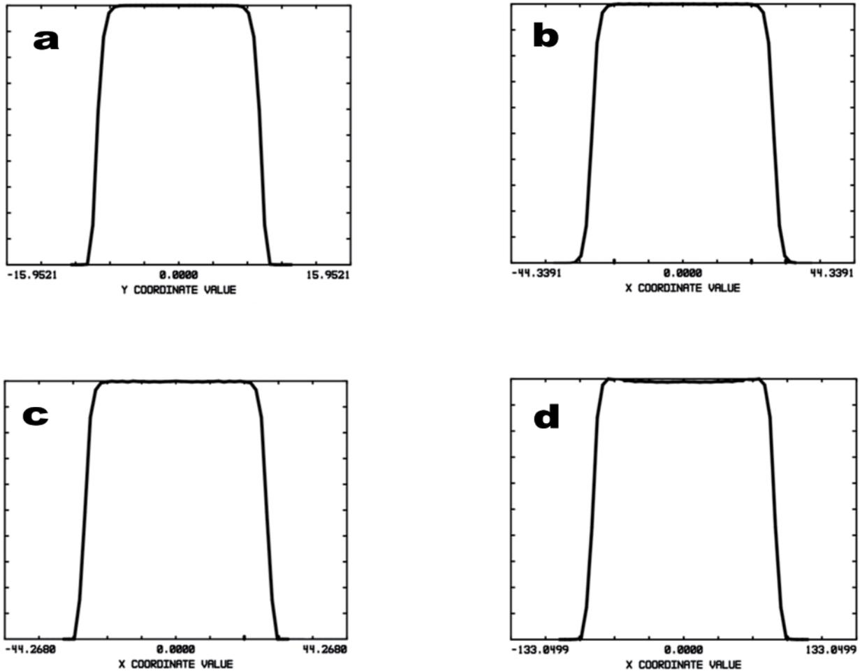
Figure 4. Beam profiles from the Zemax model of the OB system: (a) Input (b) Amplifier 1st pass (c) Amplifier 4th pass (d) First compressor grating.
