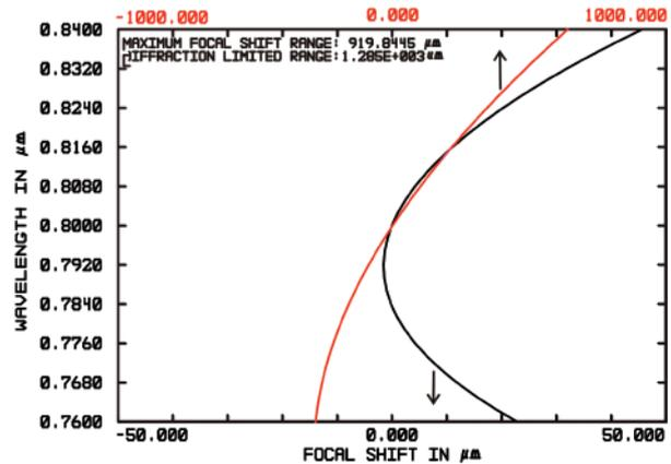
Figure 3. Comparison of focal variation of compensated (black) and uncompensated (red) beam transport systems.
