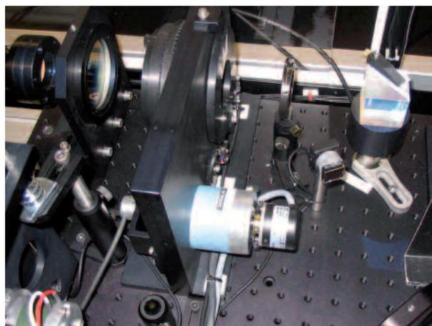
Figure 2. The optical set-up of the beam switch between TA2 and the Gemini beam line.
