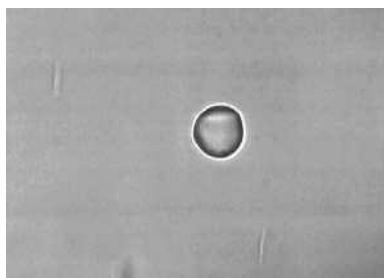
Figure 2. An image of a distorted 10 micron diameter polymer particle after polymerizing an IBA monomer droplet containing Irgacure 819 photo-initiator.
